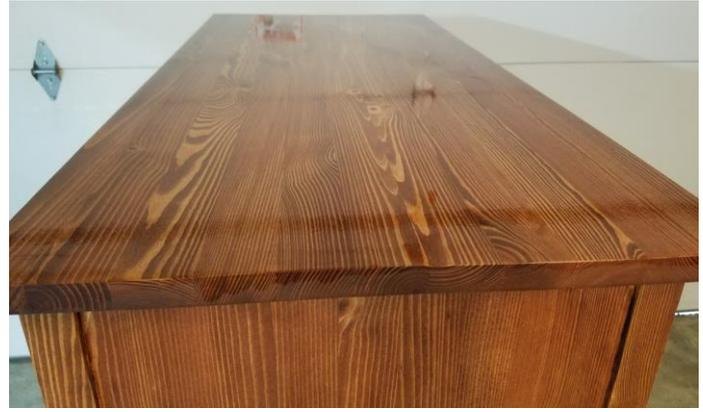
The second coat will be 9 parts polyurethane to 1 part mineral spirits. The same process will be used. Allow to dry 24 hours.
