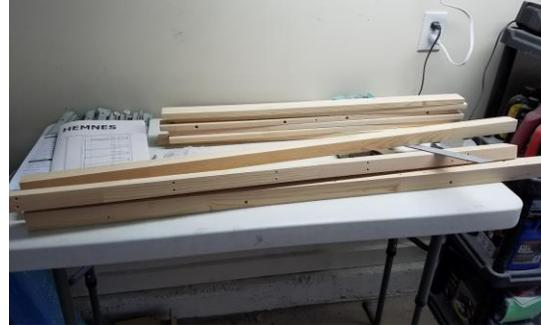
I sanded one of these before assembly and one of these after assembly. Each way has its own pros/cons but I prefer sanding before assembly as it allows you to skip certain areas that are not going to be visible (IE: the bottom of the dresser top).
